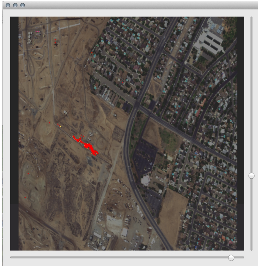
Figure 4. Screen shot of the graphical user interface, with an example of flight data from 13 June (ang20140613t184239). The red plume is displayed overprinted on RGB wavelengths.
