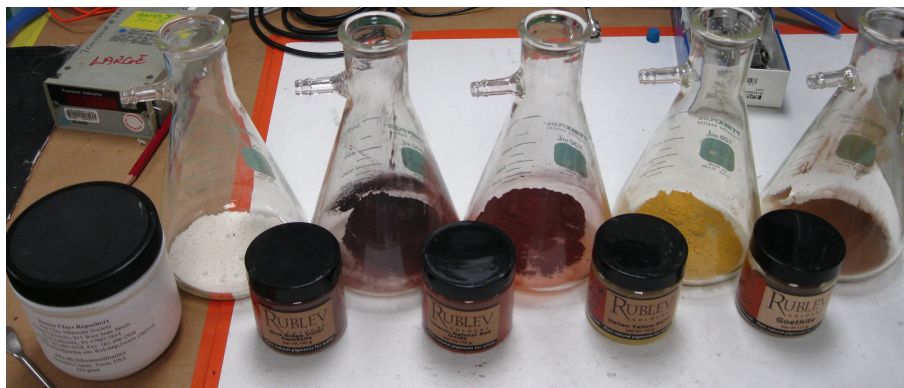
Figure 8. Pigmented dusts used in aerosol tests (from left to right: Montmorillonite, Blue Ridge Violet, Luberon Natural Red, Italian Yellow Earth, Goethite).
