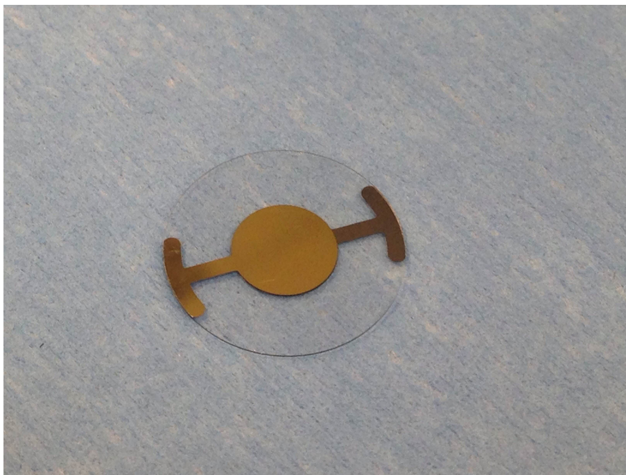
Figure 1. Piezoelectric Crystal Microbalance: quartz crystal (transparent plate) and gold electrode in the centre. On the right side and left side are presents the contact points for the proximity electronic.
