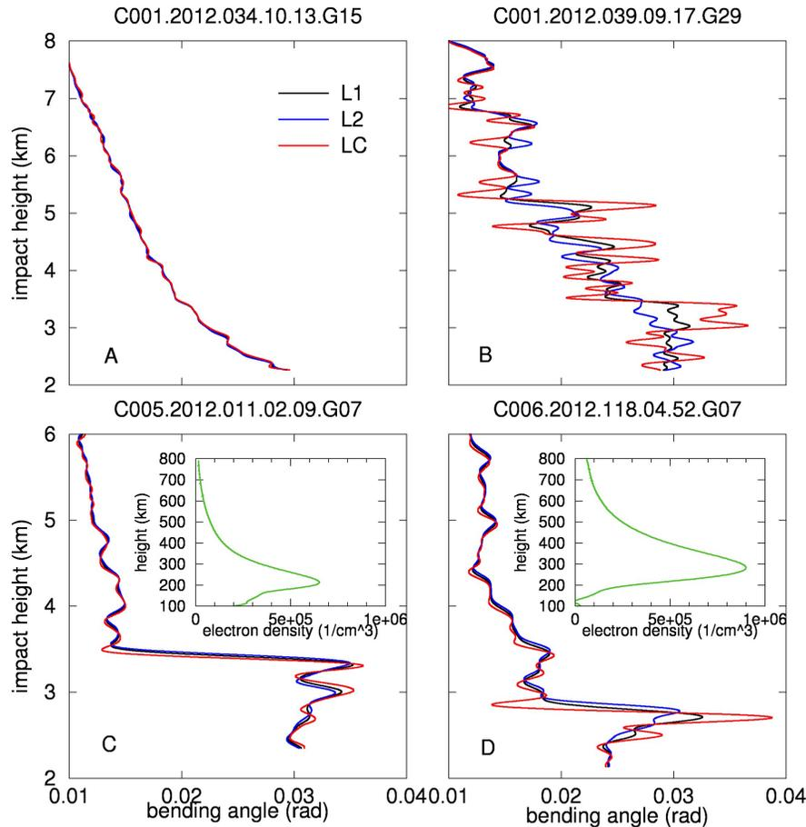
**Figure 1.** Examples of COSMIC L1CA (black), L2C (blue) and ionosphere-free (red) bending angles in the troposphere. (c and d) also include the ionosphere electron density profiles (green).
