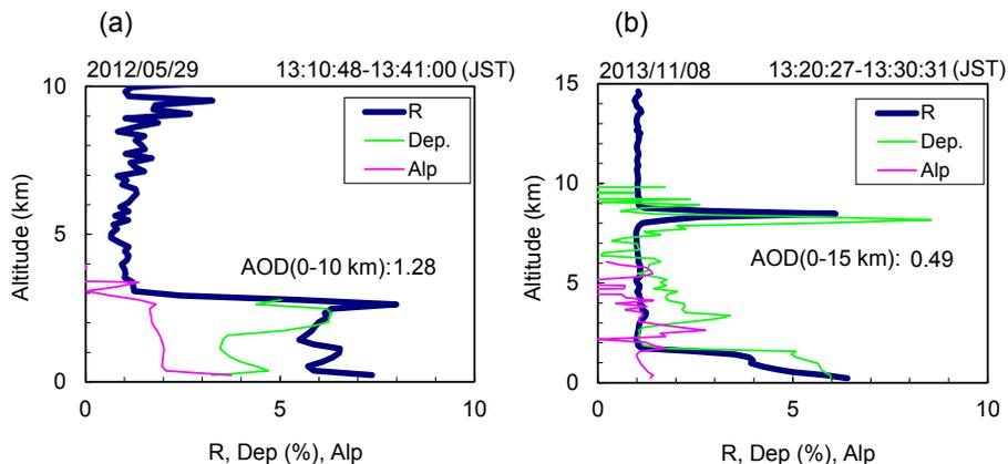
**Figure 10.** Vertical profiles of the backscattering ratio (cobalt), total depolarization ratio (green), and backscatter-related wavelength exponent (pink), measured with the Mie lidar at Saga on **(a)** 29 May 2012 and **(b)** 8 November 2013.
