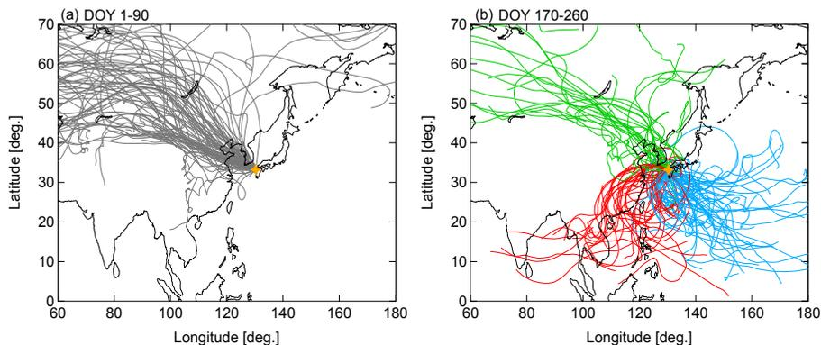
**Figure 5.** Ten-day isentropic backward trajectories from Saga at 03:00 UT on **(a)** DOY 1–90 and **(b)** DOY 170–260. The trajectories are started from an altitude of 2.6 km (approximately 700 hPa). The trajectories of DOY 170–260 are classified into three types, depending on of air mass transport, and the classification approach is described in the text.
