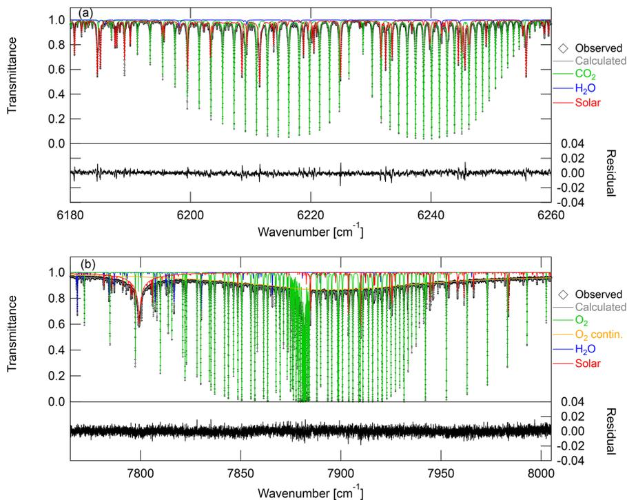
**Figure 2.** Examples of spectral fits for (a) CO<sub>2</sub> and (b) O<sub>2</sub> bands. Black diamonds denote the observed spectra on 26 November 2011, and colored lines denote the calculated spectra for the telluric and solar lines. Residuals between the observed and calculated spectra are also shown.
