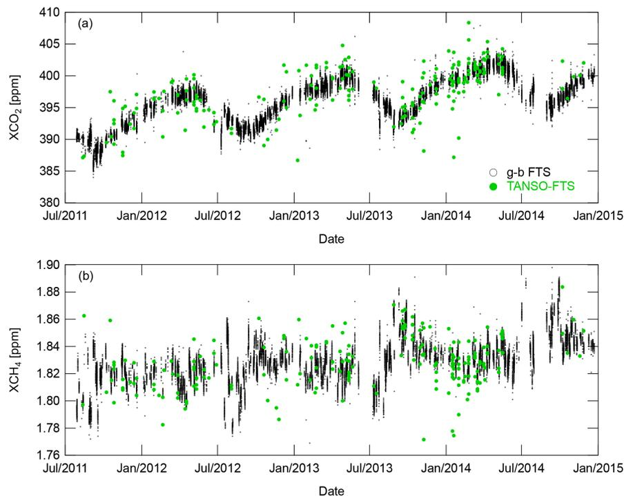
**Figure 7.** Time series of **(a)** XCO<sub>2</sub> and **(b)** XCH<sub>4</sub> for g-b FTS and TANSO-FTS data. Black circles are the g-b FTS data; green circles are the TANSO-FTS data within a  $\pm 2.0^\circ$  latitude/longitude rectangular area centered on the FTS site.
