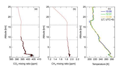
**Figure 3.** In situ (a)  $CO_2$  and (b)  $CH_4$  profiles measured by instruments onboard aircraft over the Saga FTS site on 15 January 2013. Black line represents the measured data, red line is the integrated profile (see text); dashed and dotted lines indicate tropopause height determined from NCEP reanalysis data and radiosonde temperature profiles, respectively. (c) Temperature profiles measured by radiosonde launched from Saga on 15 January 2013.
