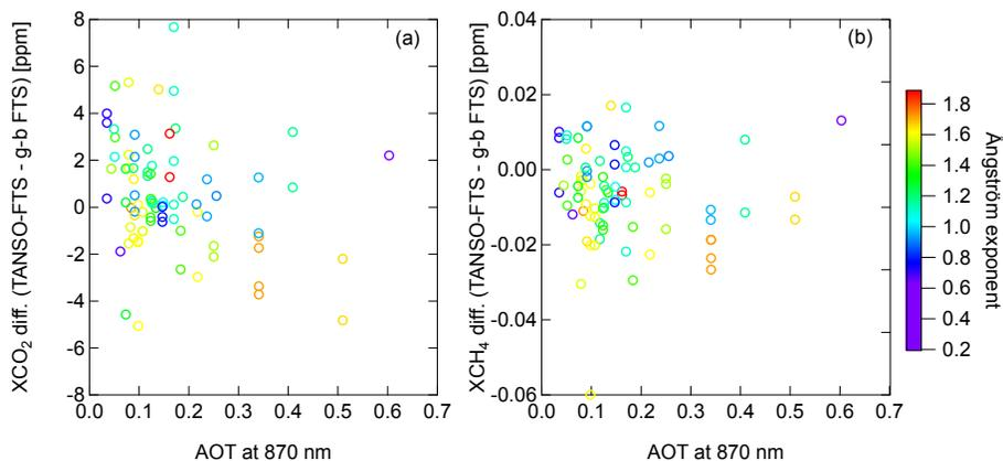
**Figure 9. (a)** Differences between XCO<sub>2</sub> values derived from TANSO-FTS and g-b FTS spectra with respect to aerosol optical thickness at 870 nm measured with the sky radiometer at Saga. Color scale represents Ångström exponent derived from the sky radiometer measurements. **(b)** Same as Fig. 9a, but for XCH<sub>4</sub> values.
