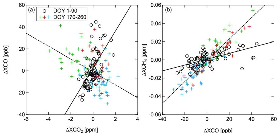
**Figure 6.** Correlation plots of **(a)**  $\Delta XCO$  and  $\Delta XCO_2$  and **(b)**  $\Delta XCH_4$  and  $\Delta XCO$ , which are represented by the differences between g-b FTS data and fitting curve values. Black circles are data for DOY 1–90; colored crosses are data for DOY 170–260. Colors correspond to those of the trajectories shown in Fig. 5b. Solid and dashed lines denote linear fits to DOY 1–90 and DOY 170–260 data, respectively.
