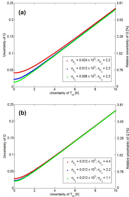
**Figure 8.** The uncertainty of the conversion factor  $Q$  as a function of the uncertainty in the mean temperature ( $T_m$ ) and for three groups of the uncertainties in the constants  $k_3$  and  $k'_2$ : the nominal value (blue line), the double of the nominal value (red line), and the half of the nominal value (green line) for **(a)** a fixed uncertainty of  $k'_2$  and **(b)** a fixed uncertainty of  $k_3$ .
