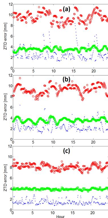
**Figure 2.** The ZTD error due to orbit errors for three GRUAN sites: **(a)** LDB0, **(b)** LDRZ and **(c)** NYA2, where the blue dots show the simulated ZTD error, the red circles show the theoretical ZTD error caused only by the radial orbit error, and the green squares show the theoretical ZTD error caused only by the tangential orbit error.
