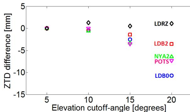
**Figure 3.** The impact of the elevation cutoff angle on the estimated ZTD for five GRUAN sites. The result obtained from the 5° elevation cutoff solution is used as the reference which however does not necessarily mean that it is the most accurate. Ideally, if all models are correct the result shall not depend on the cutoff angle at all.
