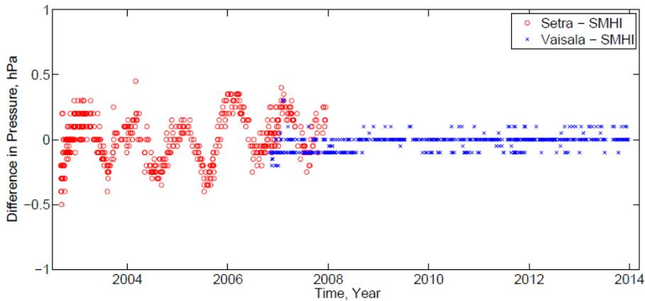
**Figure 7.** Differences in the surface pressure measured by three different barometers.
