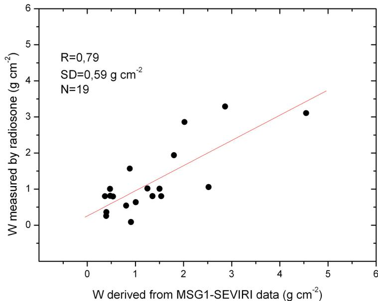
**Figure 4.** Comparison between the total atmospheric water vapor contents derived from MSG1-SEVIRI data and that measured by the radiosonde.
