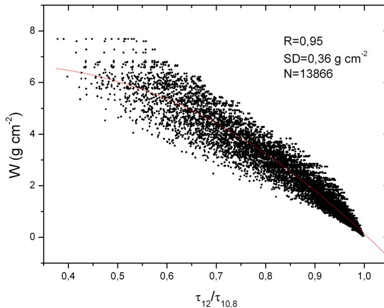
**Figure 3.** Total atmospheric water vapor content plotted as a function of the transmittance ratio,  $\tau_{12}/\tau_{10,8}$ , for MSG1-SEVIRI at different viewing angles ( $\theta = 0, 10, 20, 30, 40$  and  $50^\circ$ ).
