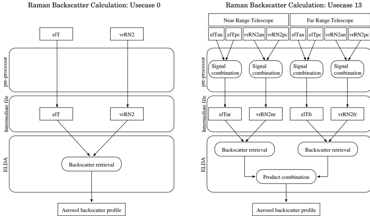
**Fig. 2.** Two examples of Raman backscatter calculation usecases implemented in the SCC. In particular the usecase 0 (on the left) can be used for a lidar system measuring only the elastic backscattered signal (eIT) and the corresponding  $N_2$  Raman backscattered signal (vrRN2). The usecase 13 (on the right) refers to more complex lidar configuration in which there are two different telescopes and each channel is acquired in both analog and photoncounting mode.
