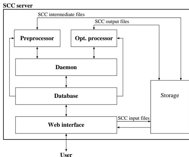
Fig. 1. Block structure of the Single Calculus Chain.
