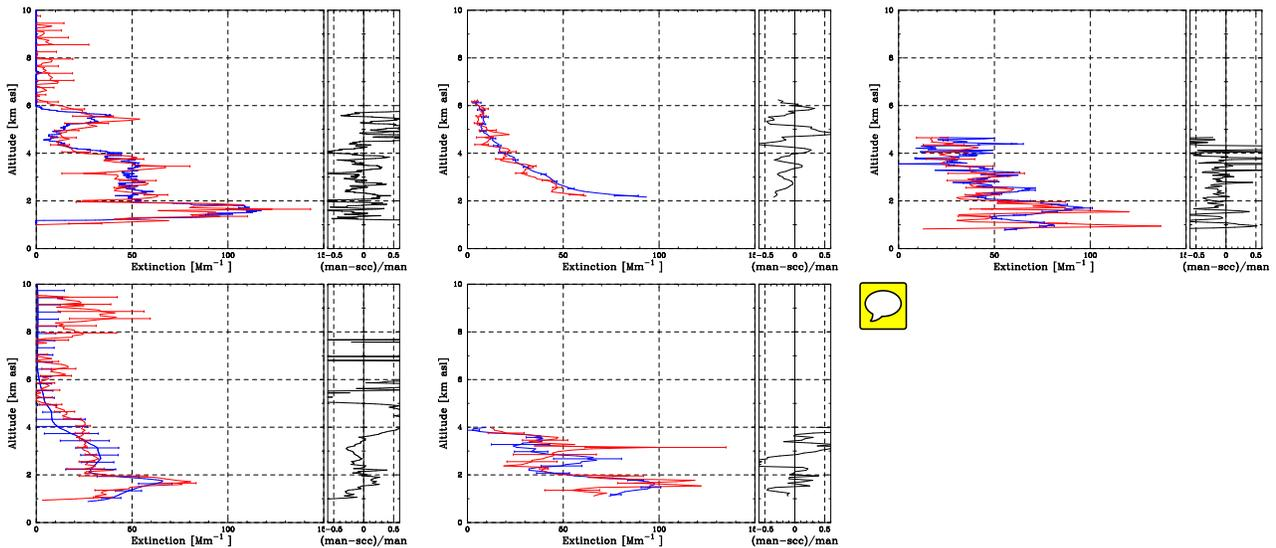
**Fig. 7.** Comparison of aerosol extinction profiles at 532nm for five lidar systems participating to the EARLI09 inter-comparison campaign. All the profiles refer to measurement session taken on 25th May 2009 21:00 to 23:00 UT and they have been retrieved using the N<sub>2</sub> Raman backscatter signal at 607nm. The profiles in blue are the analysis provided by the originator of the data using his own analysis software. The profiles in red are the ones retrieved by the SCC
