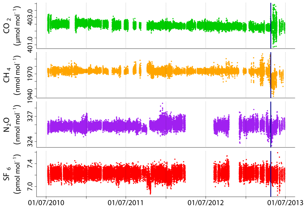
Figure 4. Time series of the target gas measured with the GC system at Puy de Dôme. The vertical blue lines on each panel correspond to the date of the working standards change.
