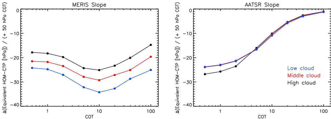
**Fig. 3.** The sensitivity of the equivalent MERIS and AATSR HOM-CTP to an increase of CGT by 50 hPa. Cloud top pressure of low cloud = 800 hPa, middle cloud = 600 hPa, and high cloud = 300 hPa.
