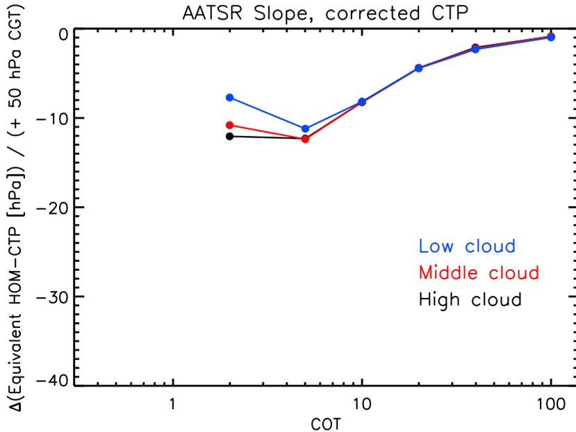
**Fig. 4.** The sensitivity of the equivalent AATSR HOM-CTP to an increase of CGT by 50 hPa. The pressure at 1 COT into the cloud is taken as corrected CTP. Cloud top pressure of low cloud = 800 hPa, middle cloud = 600 hPa, and high cloud = 300 hPa.
