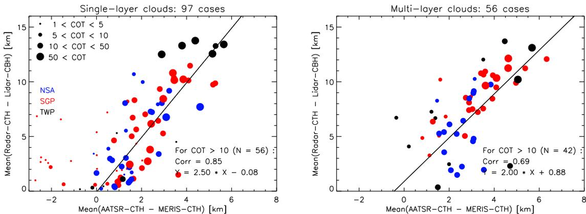
**Fig. 5.** Results of the comparison of mean cloud vertical extent derived from radar and lidar observations to the difference in mean cloud top height retrieved with AATSR and MERIS.
