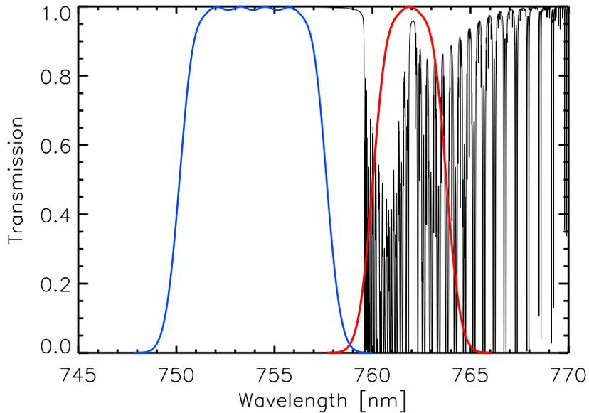
**Fig. 1.** Spectral response functions for MERIS window channel 10 (blue) and MERIS channel 11 in the oxygen-A absorption band (red). Black lines: oxygen absorption lines.
