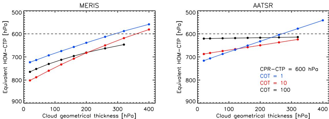
**Fig. 2.** The equivalent HOM-CTP for varying CGT and COT, assuming a CPR-cloud with CTP=600 hPa. Settings in the radiative transfer simulations: satellite viewing angle =  $0^\circ$ , solar viewing angle =  $35^\circ$ , relative azimuth angle =  $0^\circ$ , surface albedo = 0.02 and MERIS central wavelength = 762 nm.
