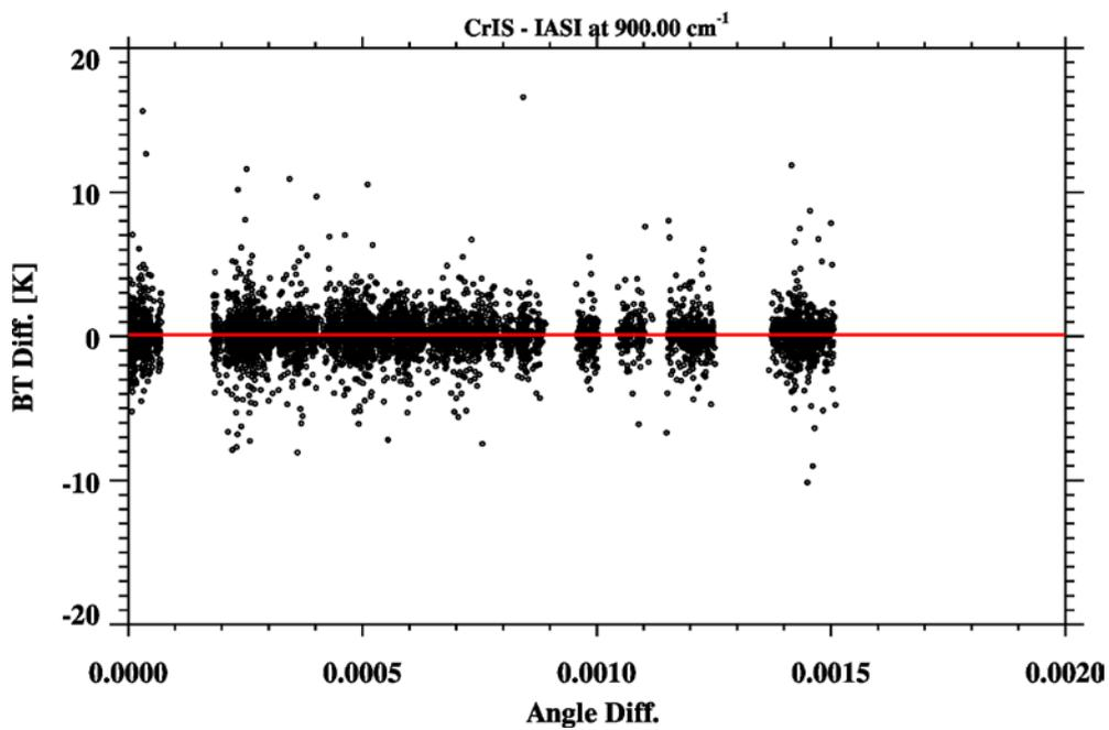
Figure R3 BT differences varying with angle distance ( $\text{abs}(\cos(\text{zen1})) - \cos(\text{zen2}))$ ) in the range from 0 to 0.002.
