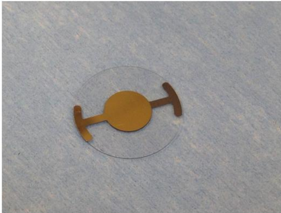
2 Figure 1. Piezoelectric Crystal Microbalance: quartz crystal (transparent plate) and gold electrode in 3 the centre. On the right side and left side are presents the contact points for the proximity electronic.
