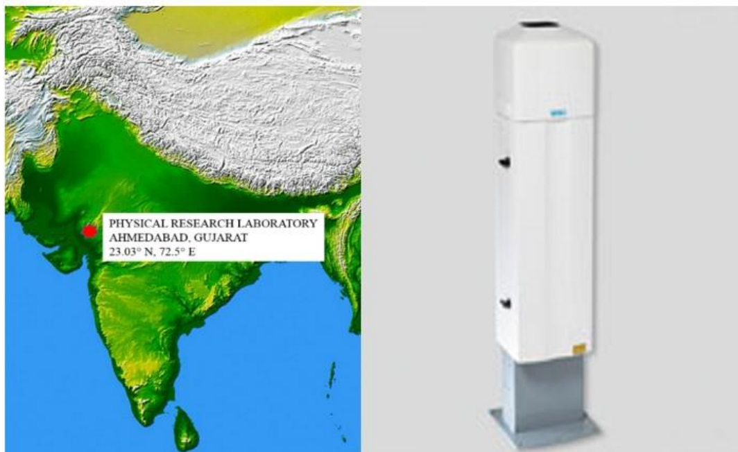
527 Figure 1. (a) Location of Ahmedabad (23° 03' N, 72° 40' E, 55 m amsl) where Ceilometer CL31 528 is installed and (b) a photograph of the Vaisala ceilometer instrument.
