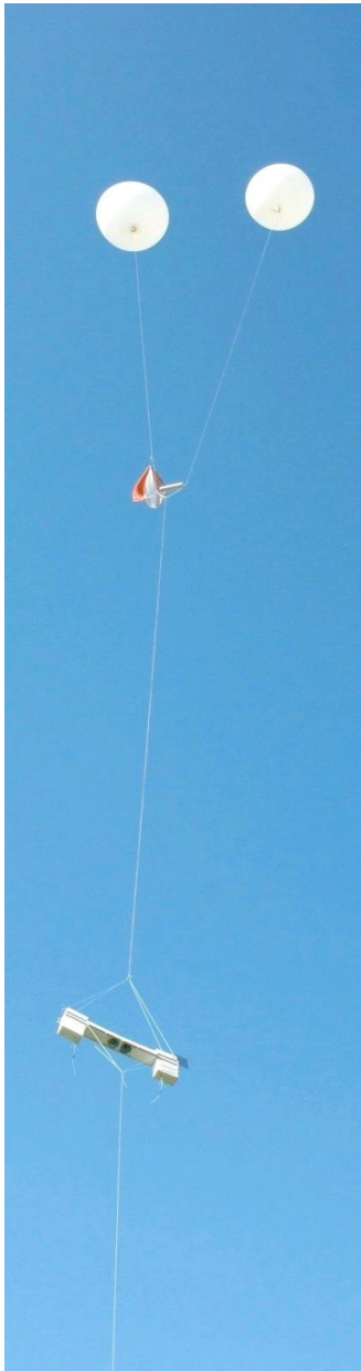
3 Figure 8: Flight configuration for the double balloon method. Each of the two balloons and 4 payload are attached to a vertex of a triangular aluminium frame outfitted with the Intelligent 5 Balloon Release Unit that releases the carrier balloon at a pre-set altitude. The configuration is 6 shown attached to the launching pole just prior to release.
