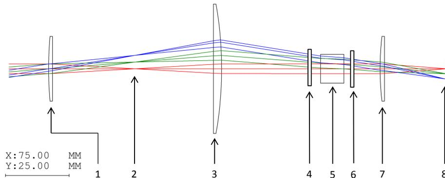
**Figure 4.** Ray Tracing diagram of the telescopic lens system for ALI simulated by Code V optical design software. The elements in the system are the following: (1) 150 mm focal length plano-convex lens. (2) Field stop. (3) 100 mm focal length plano-convex lens. (4) Vertical linear polarizer. (5) Brimrose AOTF. (6) Horizontal linear polarizer. (7) 50.4 mm focal length bi-convex lens. (8) Imaging plane.
