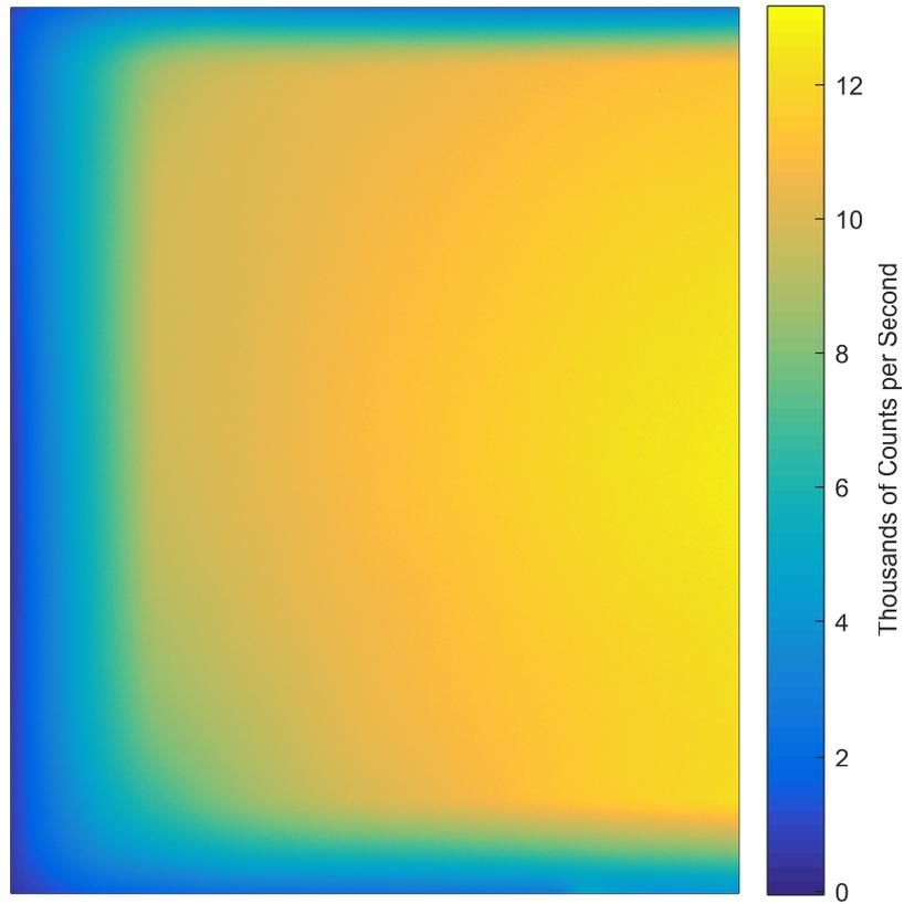
**Figure 7.** A calibration image after stray light removal has been performed where the measured wavelength is 750 nm with a 1 s exposure time. Vignetting can be seen as moving away from center of the image. Additionally the last  $1^\circ$  of the horizontal field of view ~~is~~ on the right side is lost due to strong contamination from reflections within the system.
