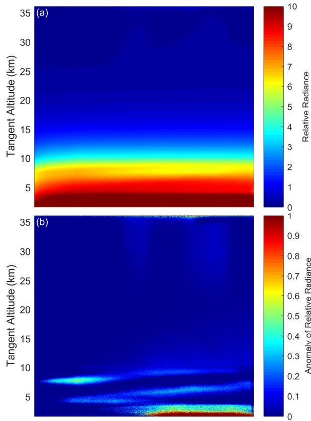
**Figure 9.** (a) Final calibrated 750 nm image, taken at 13:57 UTC located at  $48.55^\circ$  N,  $80.00^\circ$  W with a solar zenith angle and solar scattering angle of  $63^\circ$  and  $98^\circ$  respectively. (b) The same 750 nm image with the mean of the profile removed from the image leaving the residual signal that shows thin clouds in the troposphere.
