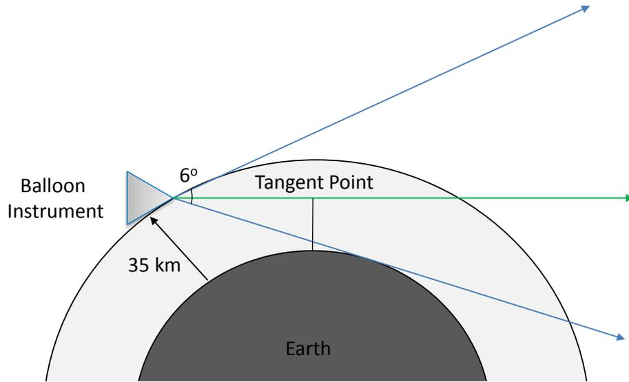
**Figure 3.** ALI in a stratospheric balloon geometry showing the complete  $6^\circ$  field of view in blue with a float altitude of 35 km. The green line shows a typical vertical line-of-sight where the tangent point or altitude is set by the minimum distance between the earth and the line-of-sight.
