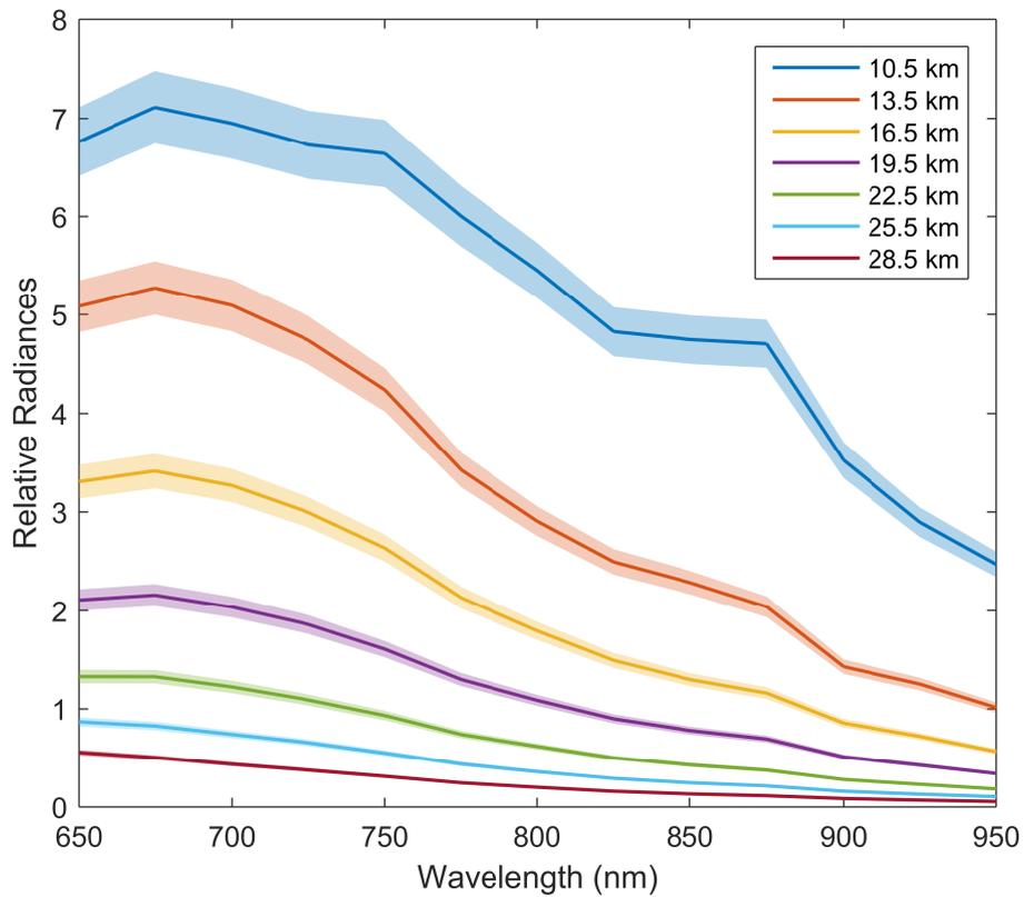
**Figure 11.** Level 1 relative radiances spectrally from 650 to 950 nm as measured from ALI at approximately 14:20 UTC consisting of images number 204 to 216 looking  $90^\circ$  in the azimuth from the sun facing southwards. These spectral profiles are presented at several tangent altitudes with a horizontal look direction of  $0^\circ$ . The shading represents the error on the radiances.
