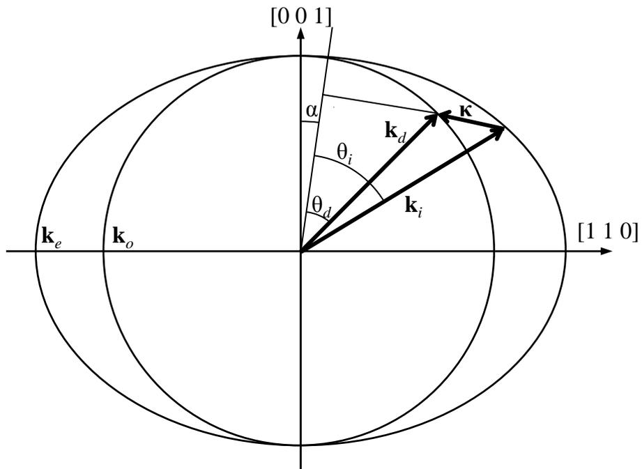
**Figure 1.** The wave vectors generated by the AOTF experiment. From Eq. (1), the incident wave vector,  $k_i$ , diffracted wave vector,  $k_d$ , and acoustic wave vector  $\kappa$  are shown. The respective interaction angles for the incident and diffracted wave vectors  $\theta_i$  and  $\theta_d$  are also presented.
