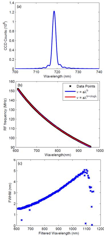
**Figure 6.** (a) A spectrum taken from the AOTF from the point spread function when the tuning frequency of the AOTF was at 124.96 MHz. (b) The calibration curves for the AOTF tuning curve which contains the data points recorded and fit curve. (c) The full width half max for each of the determined wavelengths for the AOTF. The full width half max at 600 nm is 1.5 nm and as the wavelengths get longer it increases to 4.9 nm at 1080 nm.
