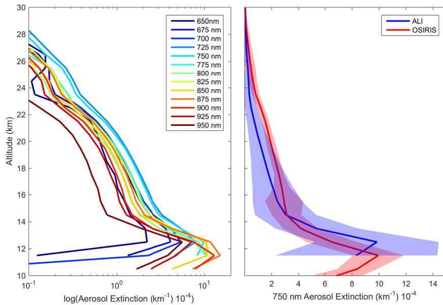
**Figure 12.** Left is the retrieved aerosol extinction profiles from the last complete imaging cycle consisting of images 205 to 216 from the 0.0° horizontal line-of-sight. Right is the 750 nm ALI aerosol extinction in blue with its error represented by the shading compared to the 750 nm extinction measured by OSIRIS in greenred with its error represented by the respective shading.
