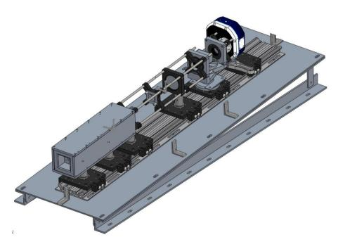
**Figure 5.** An isometric view of the complete ALI system with the baffle and 3° slant required to correctly position the field of view. Light tight case absent from diagram.
