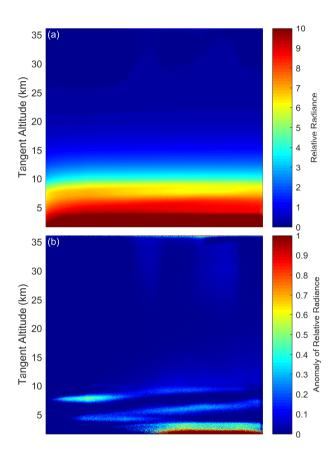
**Figure 9. (a)** Final calibrated 750 nm image, taken at 13:57 UTC located at  $48.55^{\circ}$  N,  $80.00^{\circ}$  W with a solar zenith angle and solar scattering angle of 63 and  $98^{\circ}$  respectively. **(b)** The same 750 nm image with the mean of the profile removed from the image leaving the residual signal that shows thin clouds in the troposphere.
