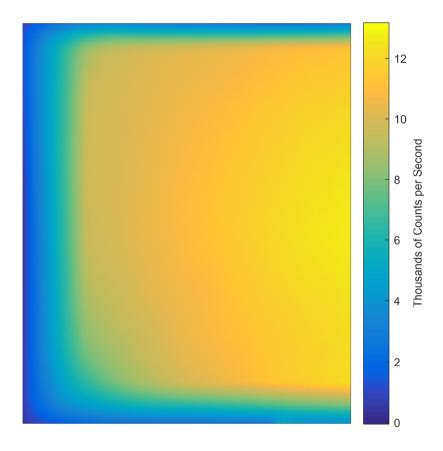
**Figure 7.** A calibration image after stray light removal has been performed where the measured wavelength is  $750 \,\mathrm{nm}$  with a 1 s exposure time. Vignetting can be seen as moving away from center of the image. Additionally the last  $1^{\circ}$  of the horizontal field of view is on the right side is lost due to strong contamination from reflections within the system.
