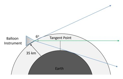
Figure 3. ALI in a stratospheric balloon geometry showing the complete  $6^{\circ}$  field of view in blue with a float altitude of 35 km. The green line shows a typical vertical line-of-sight where the tangent point or altitude is set by the minimum distance between the earth and the line-of-sight.
