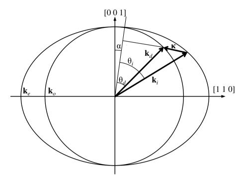
Figure 1. The wave vectors generated by the AOTF experiment. From Eq. (1), the incident wave vector,  $\mathbf{k}_i$ , diffracted wave vector,  $\mathbf{k}_d$ , and acoustic wave vector  $\boldsymbol{\kappa}$  are shown. The respective interaction angles for the incident and diffracted wave vectors  $\theta_i$  and  $\theta_d$  are also presented.
