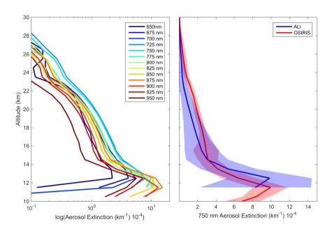
**Figure 12.** Left is the retrieved aerosol extinction profiles from the last complete imaging cycle consisting of images 205 to 216 from the  $0.0^{\circ}$  horizontal line-of-sight. Right is the 750 nm ALI aerosol extinction in blue with its error represented by the shading compared to the 750 nm extinction measured by OSIRIS in greened with its error represented by the respective shading.
