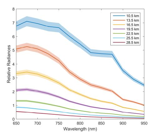
Figure 11. Level 1 relative radiances spectrally from 650 to 950 nm as measured from ALI at approximately 14:20 UTC consisting of images number 204 to 216 looking  $90^{\circ}$  in the azimuth from the sun facing southwards. These spectral profiles are presented at several tangent altitudes with a horizontal look direction of  $0^{\circ}$ . The shading represents the error on the radiances.
