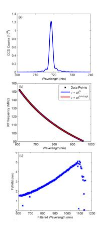
**Figure 6.** (a) A spectrum taken from the AOTF from the point spread function when the tuning frequency of the AOTF was at 124.96 MHz. (b) The calibration curves for the AOTF tuning curve which contains the data points recorded and fit curve. (c) The full width half max for each of the determined wavelengths for the AOTF. The full width half max at 600 nm is 1.5 nm and as the wavelengths get longer it increases to 4.9 nm at 1080 nm.
