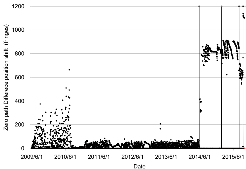
1 2 Fig. 2. Long-term ZPD position from the center of the interferogram with periodic correction 3 operations. The optical center of the interferogram is 38273 half laser fringes. The vertical 4 lines represent the time of 3 major system anomalies: solar paddle, pointing mechanism 5 change and cryocooler suspension and restart.
