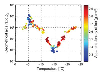
**Figure 7.** Temperature dependence of geometrical axis ratio for particles grown in the free-fall cloud chamber (Takahashi et al., 1991). Apparent density is color-coded. Note, that  $\rho_{\rm g} > 1$  corresponds to prolate particles,  $\rho_{\rm g} < 1$  corresponds to oblate particles. Numerical data were provided by Prof. Takahashi, Hokkaido University of Education, Sapporo, Japan.
