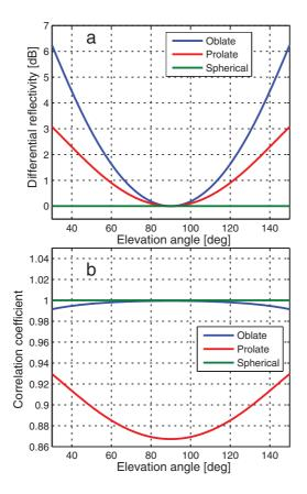
**Figure 1.** Elevation dependencies of modeled **(a)**  $Z_{\rm DR}$  and **(b)**  $\rho_{\rm HV}$  for strongly oblate (axis ratio  $\ll$  1), strongly prolate (axis ratio  $\gg$  1), and spherical (axis ratio of 1) solid ice particles. Particles are assumed to be oriented near horizontally with the degree of orientation of 0.99. The figure is based on look-up tables given in Myagkov et al. (2015b).
