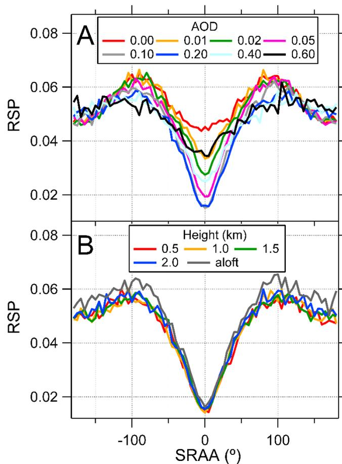
Figure R1. Sensitivity study showing that simulated RSP (430 nm) strongly influenced by (A) AOD, and insensitive to (B) aerosol vertical distribution. (A) AOD is varied, keeping aerosols homogeneously distributed (box profile) up to 1.5 km altitude. (B) The aerosol extinction
