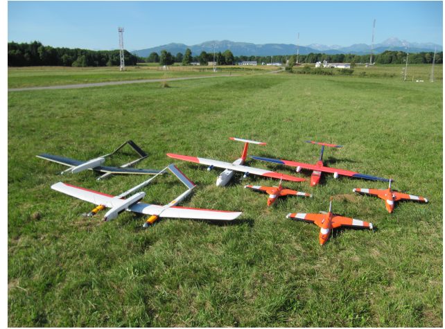
Figure 2. The fleet of RPAS operated during the whole BLLAST campaign at Site 1 in Lannemezan. From left to right: MASC (University of Tübingen), M^2AV (University of Braunschweig) and SUMO (University of Bergen). In the background the Pyrenees and the 60 m instrumented tower in the upper right corner.
