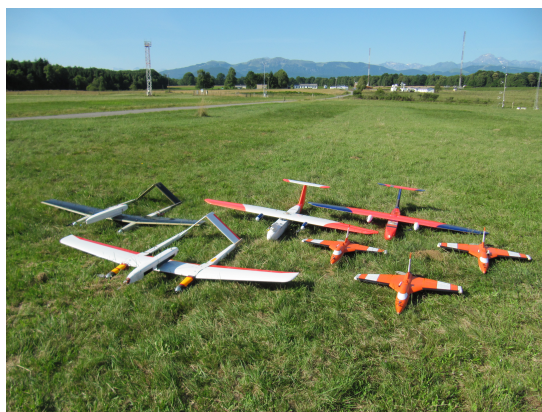
Figure 2. The fleet of RPAS operated during the whole BLLAST campaign at Site 1 in Lannemezan. From left to right: MASC (University of Tübingen), M^2AV (University of Braunschweig) and SUMO (University of Bergen). In the background the Pyrenees and the 60 m instrumented tower in the upper right corner.
