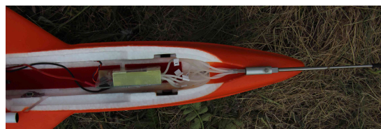
Figure 1. The 5HP and the data computer from Aeroprobe as mounted in the SUMO airframe.
