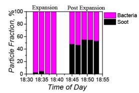
We point out that we used miniSPLAT to determine the relative soot/bacteria transmission through the IS-PCVI. miniSPLAT-measured residual counts are lower when compared to uncorrected CPC 2 counts as expected due to transmission losses in lines and detection efficiency. We note a good agreement between temporal evolution of the miniSPLAT-measured total concentration of residuals and the uncorrected CPC2 counts, which are scaled here for comparison, as shown in the figure below.
