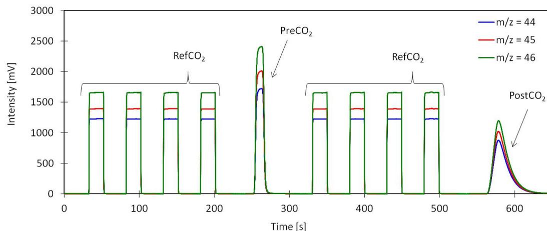
**Figure 3.** Example of a typical IRMS chromatogram of a single  $\Delta^{17}\text{O}(\text{CO}_2)$  analysis with the CF-IRMS system described here. The eight square peaks are the working reference  $\text{CO}_2$  (Ref $\text{CO}_2$ ) peaks injected directly via the open split interface. The non-equilibrated  $\text{CO}_2$  (Pre $\text{CO}_2$ ) peak and the equilibrated  $\text{CO}_2$  (Post $\text{CO}_2$ ) peak are the two sample gas peaks.
