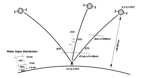
Figure 3. Schematic presentation of individual Slant Total Delays (STDs) from 3 GNSS satellites and their mapping to Zenith Total Delay (ZTD).
