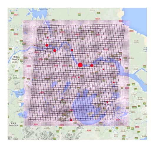
**Figure 1.** Target area showing the geoCARB footprints (skewed grid) and the centres of the Weather Research and Forecasting model cells (small red dots). The large red dots indicate power stations as listed by CARMA (2012), with the sizes of the dots proportional to the annual  $CO_2$  emissions from the plants. The distance from the south-west to the south-east corner of the geoCARB grid is approximately 158 km, while from the south-east to the north-east corner is approximately 176 km.
