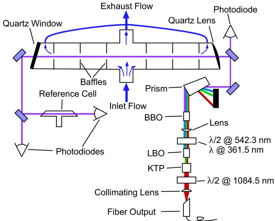
**Fig. 1.** New Figure 4: Schematic of the free space beam.
