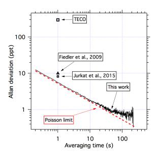
Figure 11: Instrument precision (Allan deviation) during a 1.2 hour segment sampling an average SO<sub>2</sub> abundance of 3.1 ppt in the LS during the Oct. 28 flight compared to the expected precision (Poisson limit). Other points show 1-σ precision values for a commercial pulsed-fluorescence instrument (TECO) and two CIMS instruments (Jurkat et al., 2015; Roiger et al., 2011).
