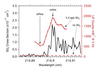
Figure 9: Example of observed signal during a scan of the laser when sampling 3.4 ppb SO<sub>2</sub> from a gas standard during a WB-57F flight. The black line plotted on the left axis shows the literature SO<sub>2</sub> absorption cross section. Plotted in red against the right axis is the observed signal from the LIF system. Red dash line shows typical signal observed when scanning laser with a zero-air sample.
