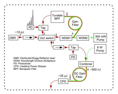
Figure 3: Schematic of the fiber-amplified diode laser system at 1084.5 nm. See text in Section 2.2 for detailed explanation.
