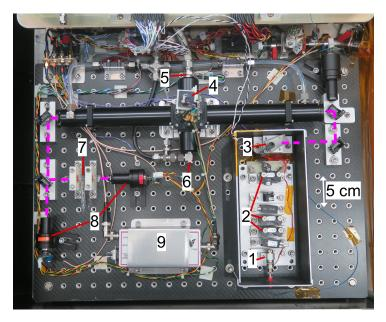
Figure 4: Optics bench photo. Dashed pink line indicates 217 nm beam path. Labeled parts: 1) fiber output, 2) nonlinear crystals, 3) Pellin-Broca prism, 4) PMT, 5) sample inlet, 6) main exhaust, 7) SO<sub>2</sub> reference cell, 8) Photodiodes, 9) PAD.
