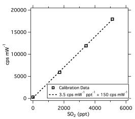
Figure 7: Example in-flight SO<sub>2</sub> calibration during the flight of October 28, 2015. Data shown are the linearized count rate divided by the measured laser power. The dashed line shows a fit to the 4 data points indicating the sensitivity of 3.5 cps / mW / ppt and background of 150 cps / mW.
