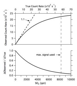
Figure 5: Count rate linearity adjustment. (Top) Calculated relationship between observed and true photon count rates from Eq. (1) assuming a 25 kHz laser pulse frequency and a maximum of 1 count / laser pulse. (Bottom) Fraction of increased signal observed as a function of the true count rate (O). Bottom axis (SO<sub>2</sub>) is calculated from the top axis assuming 300 cps background and 7 cps / ppt signal.
