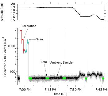
Figure 10: Data sample from flight on Oct. 27, 2015. Top panel shows ambient pressure, indicating a cruise in the lower stratosphere followed by descent into the upper troposphere. Bottom panel: Gray shows 5 Hz data. Black, red, cyan and green show 1 Hz averages of ambient sampling, calibration, laser wavelength scan, and zero-air zeroing.
