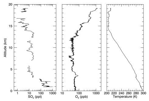
Figure 12: Data from final descent on Oct. 28. Left panel: 10 s averages shown above 3 km, 1 s averages shown below 3 km. Gaps 10 in the SO<sub>2</sub> data are during periods where instrument calibrations and zero measurements occurred.
