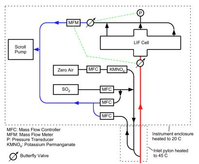
Figure 6: Schematic of flow and calibration system. Red line indicates the main inlet, which was housed in a pylon extending 28 cm below the WB-57F skin, and heated to 45 °C. Blue lines indicate components at vacuum (< 5 hPa). Excluding the components in the inlet pylon, all instrument components were housed in an insulated enclosure maintained at 20 - 30 °C.
