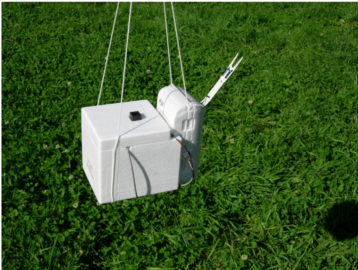
Figure 2. Photograph of the CPS within its flight package (with a black inlet duct on top) connected to the Meisei RS-11G radiosonde (with the temperature and RH sensor boom). The three 3-V lithium batteries and the interface board are placed within the CPS flight package.
