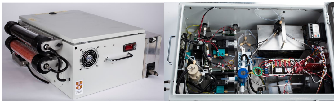
Figure 2. The exterior (2a) and interior (2b) of the new and portable Online Particle-bound ROS Instrument (OPROSI). All components shown are attached and integrated into, or onto, a portable box (60 x 50 x 25 cm) to allow easier deployment for field studies.
