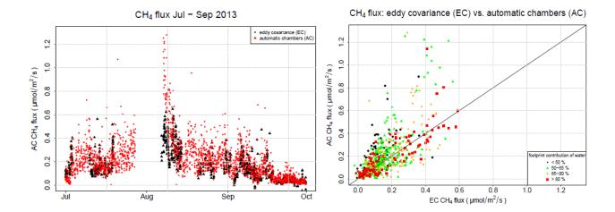
" $CH_{4_{\rm total}}$  fluxes observed by the AC system and calculated with the presented algorithm were comparable to  $CH_4$  emissions measured during the study period by a nearby eddy covariance system (Franz et al. 2015)."
