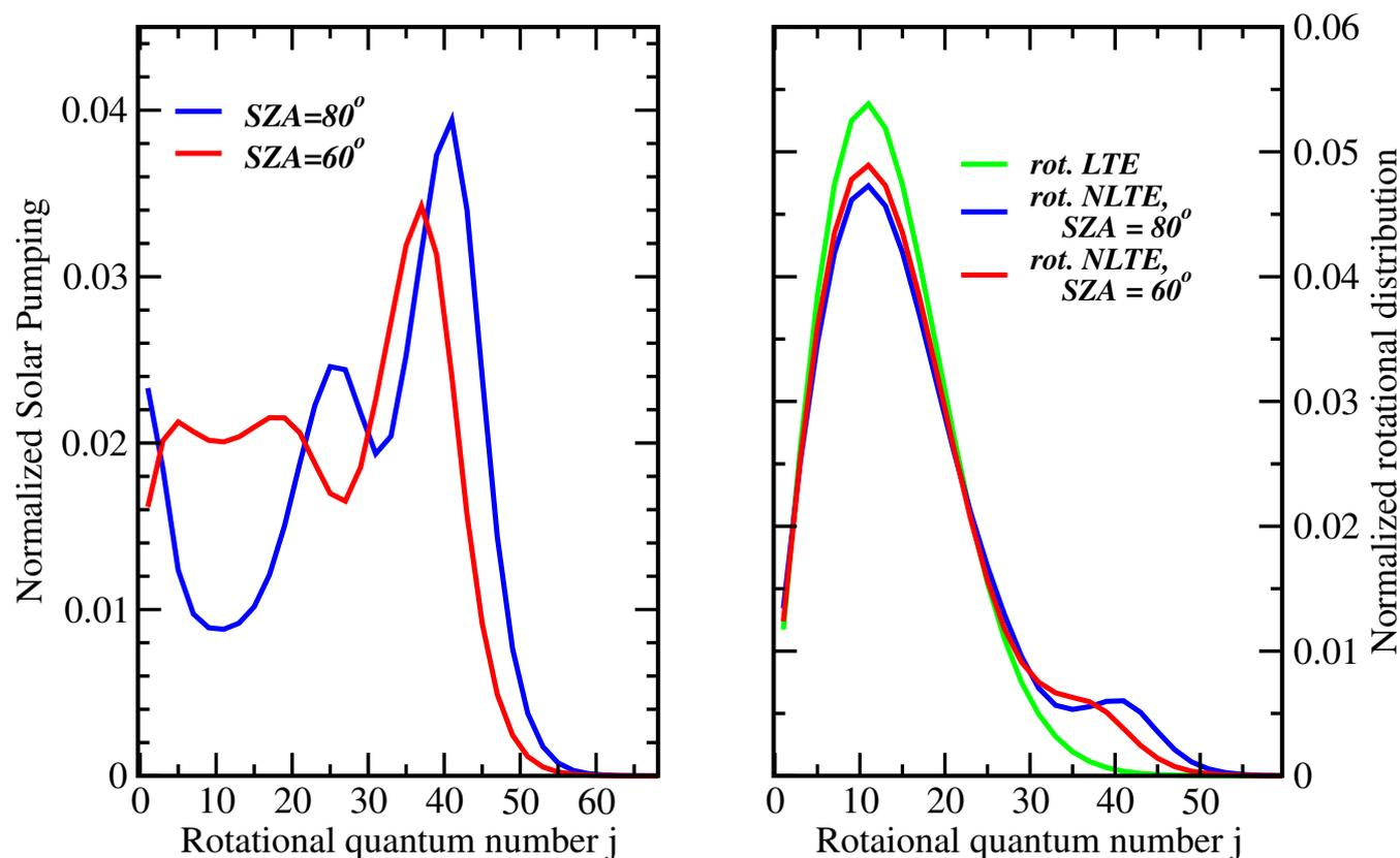
**Figure 2.** Left - normalized distribution of radiative pumping at level 10011 of  $^{12}\text{C}^{16}\text{O}_2$  due to the absorption of the  $2.7 \mu\text{m}$  solar radiation, altitude 100 km. Right - normalized rotational distribution at level 10011 of  $^{12}\text{C}^{16}\text{O}_2$ , altitude 100 km
