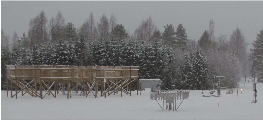
Figure 1. Snow precipitation instruments on the measurement field in Hyttiala . The Pluvio 2 200 is inside the wind protection on a platform and the PIP lamp can be seen at right on the ground. The view of the picture is to southwest and the distance from the platform to the treeline behind is approximately 20 m.
