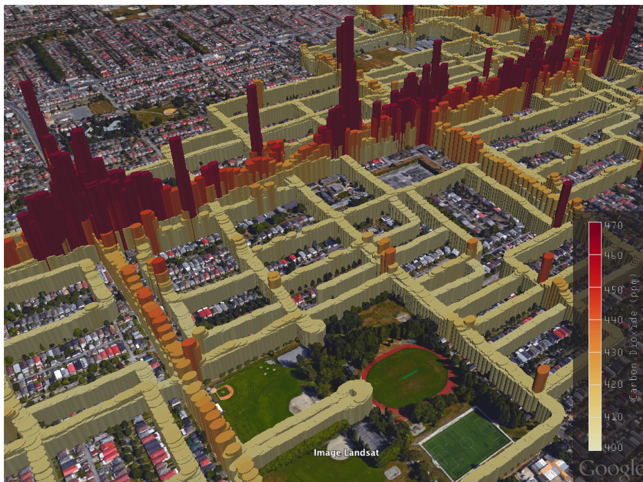
Figure 4. 3D-visualization of all raw r_{\text{mobile}} measurements from all systems (summer campaign) in the “Sunset / Victoria-Fraserview” neighborhood. The visualization is illustrating the high density of measurements taken along streets, laneways, and in parks. The linear area with many higher mixing ratios is the busy 6-lane “Knight St”. with \approx 50,000 vehicles per day. Image visualized in Google Earth.
