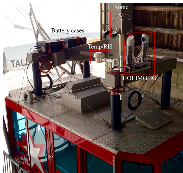
Figure 1. Experimental set up of the HoloGondel platform during the measurement campaign at the Eggishorn in the winter season 2016/2017. The picture was taken in the lower station of the cable car in Fiescheralp. The GPS Sensor is not visible on this picture, because it is mounted on the opposite side of the crossbar.
