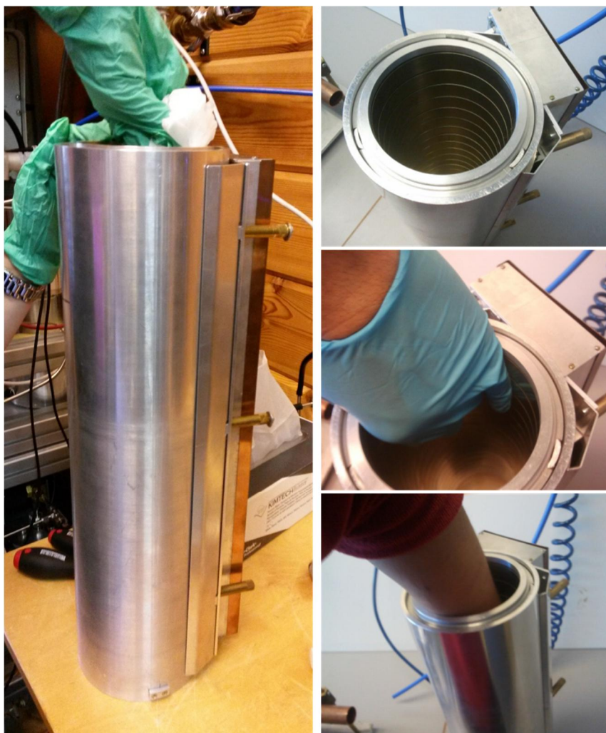
Fig. 11. Cleaning electrometer rings by opening the mobility analyser and wiping with clean cloth.
