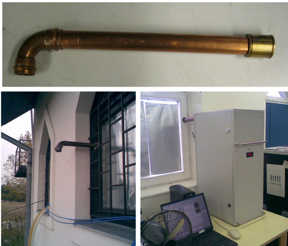
Fig. 7. Example an aerosol sampling inlet for the NAIS used at K-puszta, Hungary. A grid is missing in the top figure from the end of the sampling line. Below it is seen in an instrument set-up on field.
