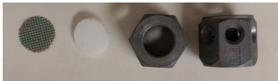
**Figure 1.** PAM reactor “inlet mixer”. A mesh screen or Teflon disc is press fit into a nut with drilled-out holes to promote axial mixing.
