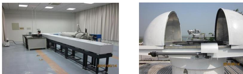
Figure 2. Bruker IFS 125HR spectrometer (left panel) and solar tracker (right panel).
