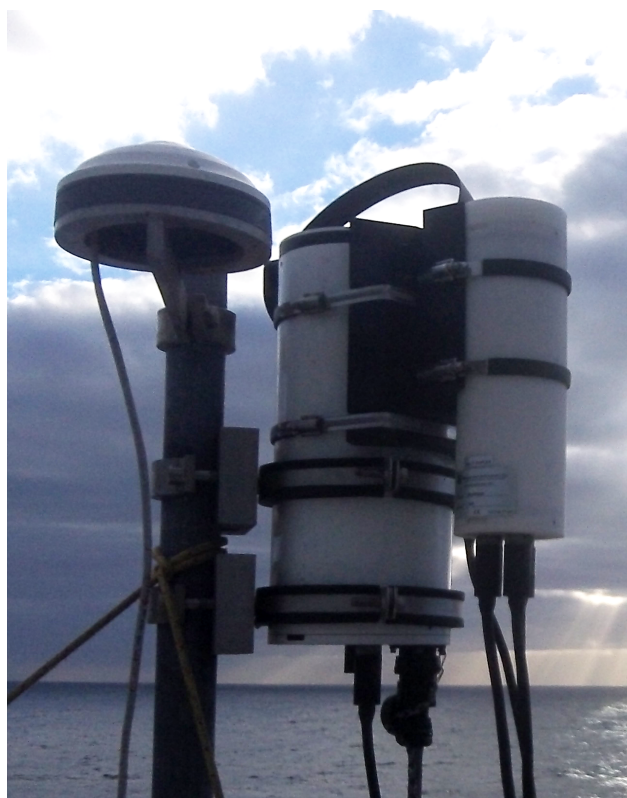
Figure 1. The shadow band radiometer GUVis mounted on the research vessel Polarstern during the cruise PS83 together with a total-sky imager.
