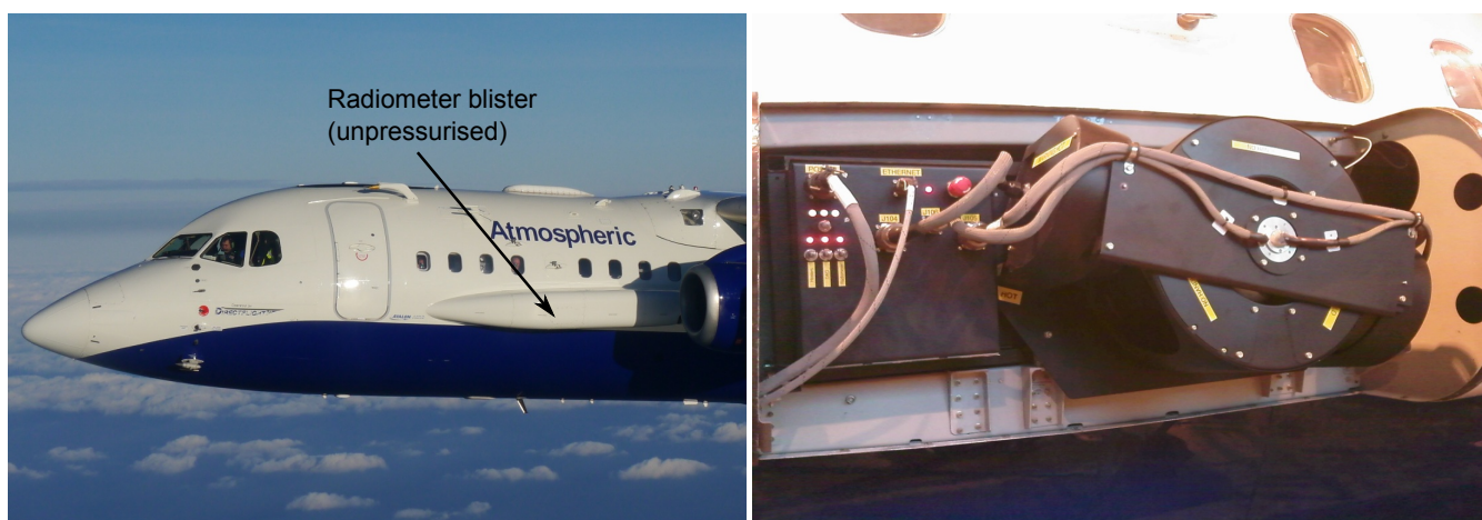
Figure 1. The location of the radiometer blister on the FAAM BAe-146 aircraft, and the ISMAR instrument installed in the blister with the cover removed
