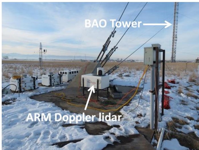
Figure 1: a) Setup of the ARM Doppler lidar, and b) aerial view showing the location of the lidar relative to the BAO tower during XPIA.
