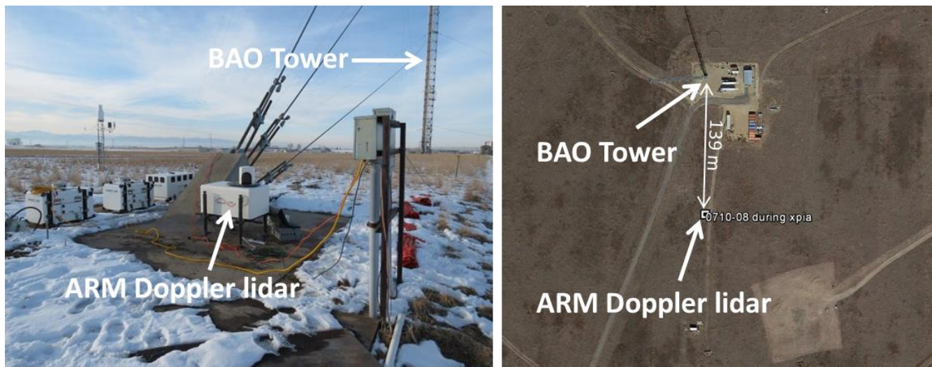
Figure 1: a) Setup of the ARM Doppler lidar, and b) aerial view showing the location of the lidar relative to the BAO tower during XPIA.
