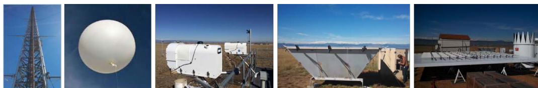
635 Figure 1: Instruments used in this study. From the left: 300-m equipped meteorological 636 tower (photo credit: Katie McCaffrey), radiosonde, 2 MWRs, 915-MHz and RASS system 637 (photo credit: Katie McCaffrey), 449-MHz and RASS system (photo credit: Katie 638 McCaffrey).
