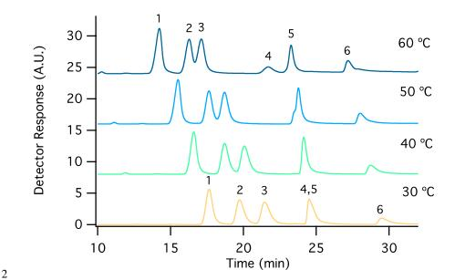
Figure 2. Separation of 1  $\mu$ g ml<sup>-1</sup> mixed amines standard with the final method gradient elution program at 30 °C, 40 °C, 50 °C and 60 °C. The peak elution order was MMAH<sup>+</sup> (1), MEAH<sup>+</sup> (2), DMAH<sup>+</sup> (3), TMAH<sup>+</sup> (4), DEAH<sup>+</sup> (5), and TEAH<sup>+</sup> (6). The separation of diethylamine (DEA) from trimethylamine (TEA) was achieved at column temperatures greater than 50 °C.
