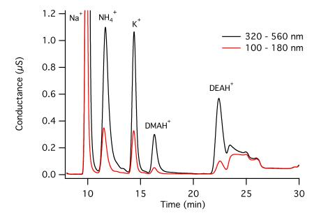
Figure 4. Overlaid chromatograms of MOUDI size-fractionated particle samples collected in St John's on July 6, 2013 during the intrusion of a biomass-burning plume that originated from Northern Labrador and Quebec. The robustness of the separation method for MMAH $^+$ , DMAH $^+$  and DEAH $^+$  from the common inorganic cations is demonstrated for the 320-560 nm (Black) and 100-180 nm (Red) size bins.
