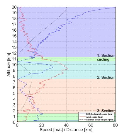
Figure 9: Wind Speed analyses from a flight from 20 km altitude. Three sections of very different wind speed and horizontal flight speed are shown. Wind speeds of up to 41 m/s and horizontal flight speeds of more than 80 m/s were recorded. The circling down happened in two phases. The black dotted curve shows the distance to the landing site.
