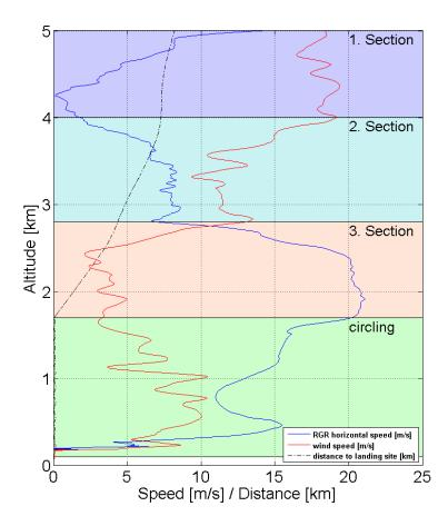
Figure 8: Wind Speed analyses from a flight beginning at 5 km altitude. Three sections of very different wind speed and horizontal flight speed occur. Wind speeds of up to 19 m/s and horizontal flight speeds of more than 20 m/s were recorded. The circling down is through moderate wind speed. The black dotted curve shows the distance to the landing site.
