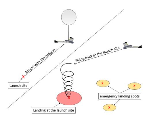
Figure 1: Schematic of ascent with the balloon (left), and descent with the RGR flying back to the launch site (right)
