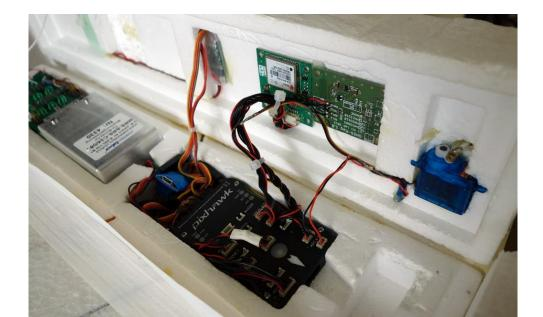
Figure 5: Upper compartment of middle payload section showing the PIXHAWK autopilot in the front part of the main box and the radiosonde module in charge of all the measurements behind. From left to right in the cover of the upper compartment: balloon release mechanism, two GPS/GLONASS modules, servo for parachute release
