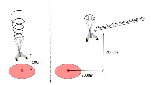
Figure 2: Schematic of landing procedure after successfully reaching the landing site by releasing the parachute 100 m above the ground (left). An emergency landing is performed by releasing the parachute when not reaching the desired landing coordinates or in any emergency situation (right).
