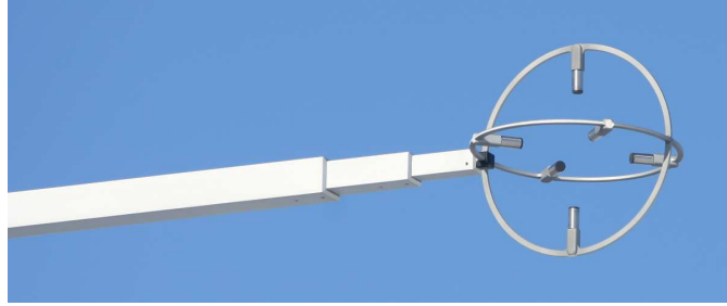
Figure 1. Photograph of the sonic anemometer used for TILDAE. The sensor head (right) incorporates six transducers, which are mounted in the cylindrical housings that protrude inward from the metal rings. The effective distance between oppositely positioned transducers is approximately 10 cm.
