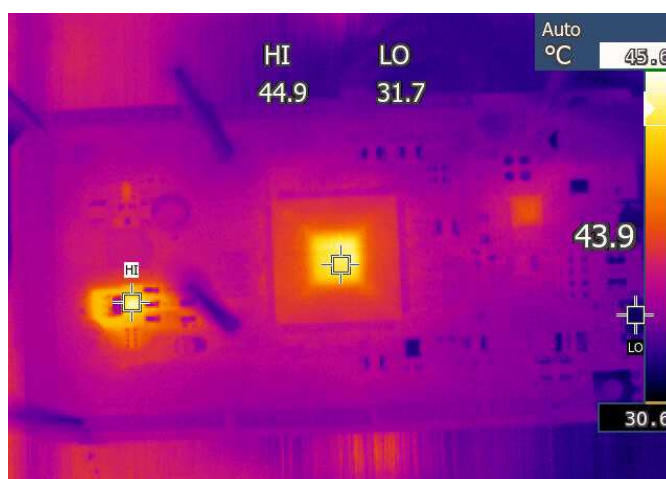
Figure 5. Thermal image of the Arduino Due during operation.
