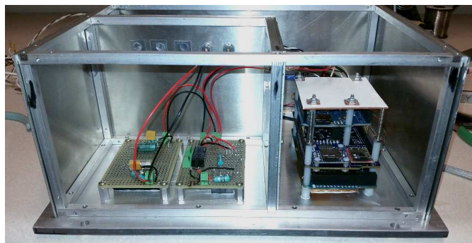
Figure 4. Photograph of TILDAE's electronics box with some of its panels removed. The power supply is visible on the left, and the microcontroller "stack" on the right.
