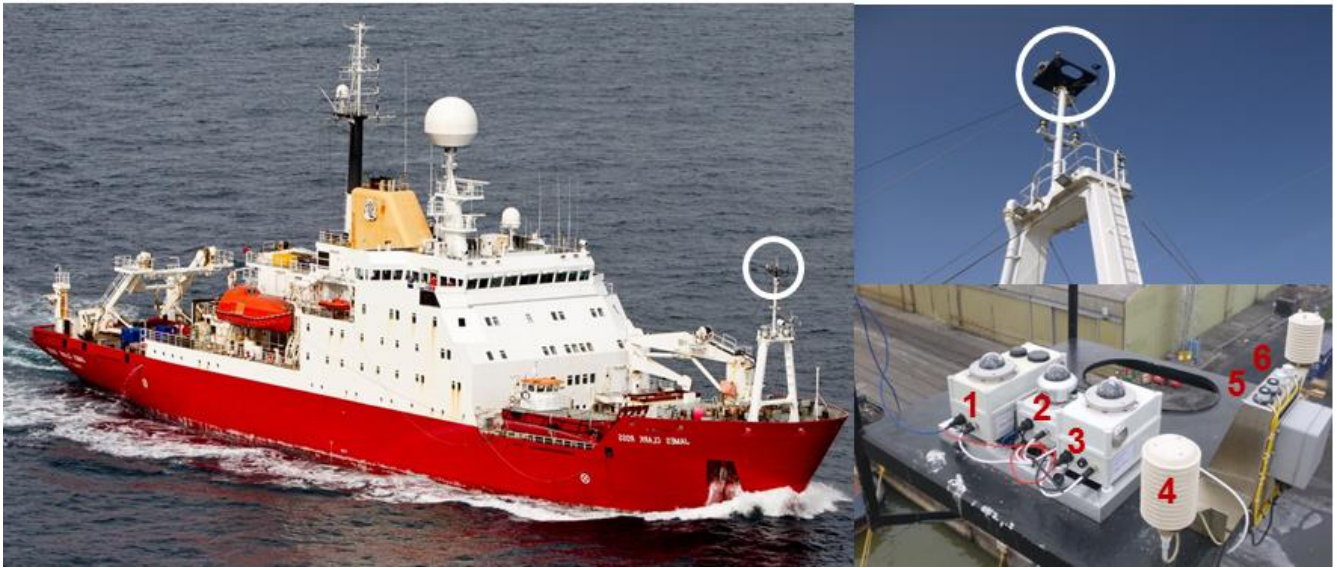
Figure 3: Main image - RRS James Clark Ross showing the position of the foremast and instrument platform (circled). Top right: The instrument platform (circled) viewed from below on the main-deck. Bottom right: instruments in situ on the platform. (1) Spectrometer 1 – AS161; (2) SPN1; (3) Spectrometer 2 - Zeiss; (4) meteorological instrument solar radiation shield; (5) Kipp & Zonen PAR sensors (x2); (6) Kipp & Zonen pyranometers (x2).
