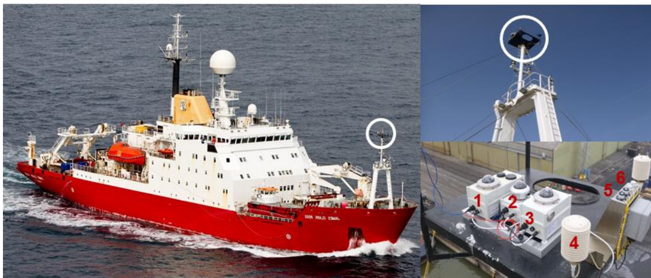
5 Figure 3: Main image - RRS James Clark Ross showing the position of the foremast and instrument platform (circled). Top right: The instrument platform (circled) viewed from below on the main-deck. Bottom right: instruments in situ on the platform. (1) Spectrometer 1 – AS161; (2) SPN1; (3) Spectrometer 2 - Zeiss; (4) meteorological instrument solar radiation shield; (5) Kipp & Zonen PAR sensors (x2); (6) Kipp & Zonen pyranometers (x2).
