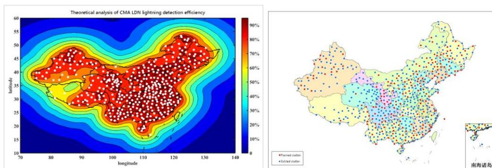
Fig.1 Left is theoretical distribution map of detection efficiency, right is CMA LDN station
